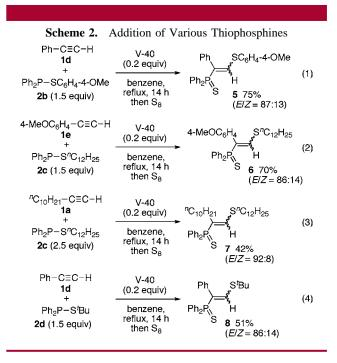
Alkylthiophosphine **2c** as well as arylthiophosphines **2a** and **2b** reacted with terminal alkynes (eqs 2 and 3). The addition of **2c** to alkyl-substituted alkyne **1a** was less efficient (eq 3). The reaction of phenylacetylene (**1d**) with bulky (*tert*-butylthio)diphenylphosphine (**2d**) proceeded to afford the adduct **8** in moderate yield (eq 4).
